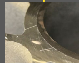
Scratches on the deck face
